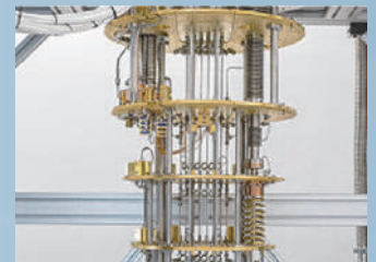
Inside the dilution refrigerator of OQC's quantum computing hardware
