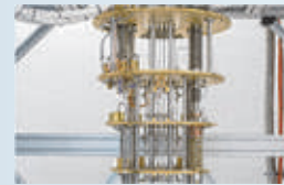
Inside the dilution refrigerator of OQC's quantum computing hardware
