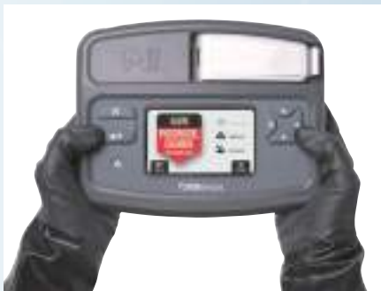
M908 : World's First Handheld Mass Spectrometer.
