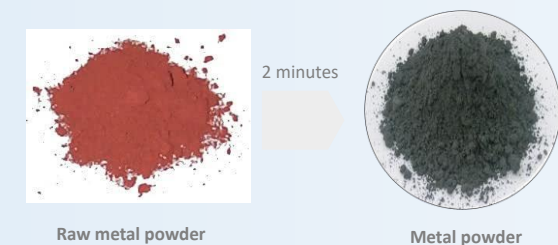
In-situ production of metal powder from raw metal powder (CO2-free)
