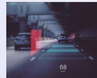
AR HUD, one of the applications of VividQ software, superimposes information in a form that matches the object in the real world
