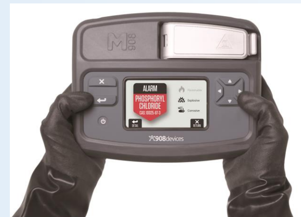
M908 : World's First Handheld Mass Spectrometer.
